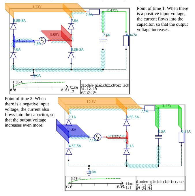
Conclusion: The output voltage over the capacitor increases until the output voltage reaches an equilibrium value, which is circa the peak of the ac input voltage.
